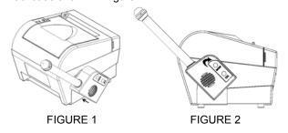
Step 2: Rotate the Main Unit clockwise as shown in figures
