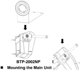
Step 1: Insert the Main Unit in the plastic turn-plate of the Bracket as shown in Figure 1.
